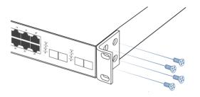
2 Secure the mounting brackets to an EIA standard size (19") rack.
